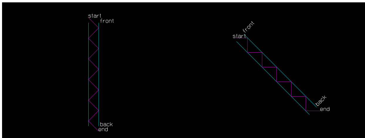
Fig. 121.4. Zigzag amplifier consisting of two mirrors, shown in the gain coordinate system. A configuration of ten reflections is shown. The start and end of the center ray is indicated as well as the front and back of the zigzag amplifier. For this case, the ray enters the front.
