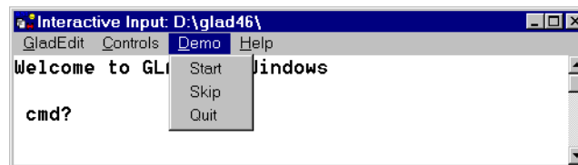
Fig. 1.9. The Demo menu item runs preselected examples. Select Start to begin the demo, Skip to skip to the next example, and Quit to end the demonstration. See Demo.pdf in the installation folder for a description of the examples.
